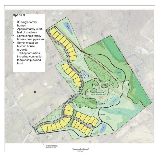
CCPC Alternative Sketch Plan – Option C (Base drawing from sketch plan prepared by D.L. Howell & Associates, Inc., dated 11/10/2020)
