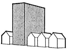
CONSIDER - Relating the overall height of new construction to that of adjacent structures. As a general rule, construct new buildings to a height roughly equal to the average height of buildings on or across the street.
